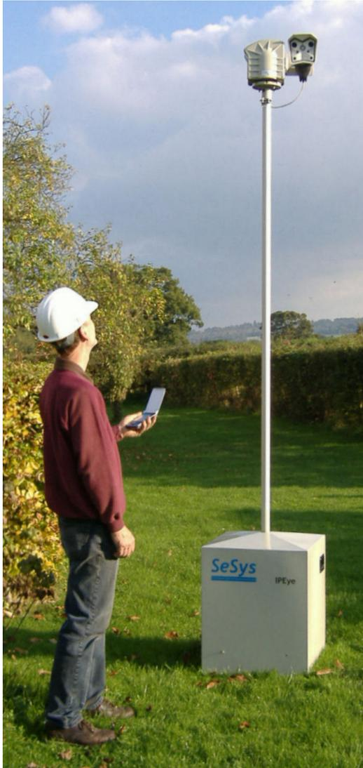
The system utilises an advanced web enabled camera, which can transfer images to the Internet either in a scheduled manner or event controlled using one of a number of built-in sensors. Event controlled image recording can be triggered using separate sensor inputs, motion detection windows, passive infrared (PIR) sensor or noise sensor via the camera's built-in microphone.
